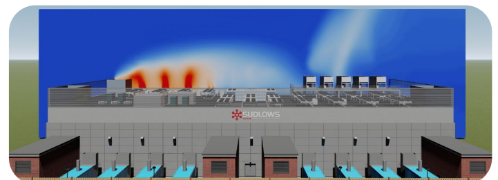
Temperature plane through the heat rejection systems displaying high levels of recirculation where equipment air flow is constrained or hindered by the air flow over and around the building
